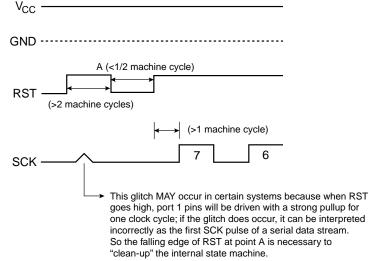
These waveforms should be used in addition to the serial downloading waveforms shown in the respective device datasheets.
